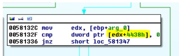
First 4 bytes of our packet are not equal to zero, so we jump to loc\_581347 function;
