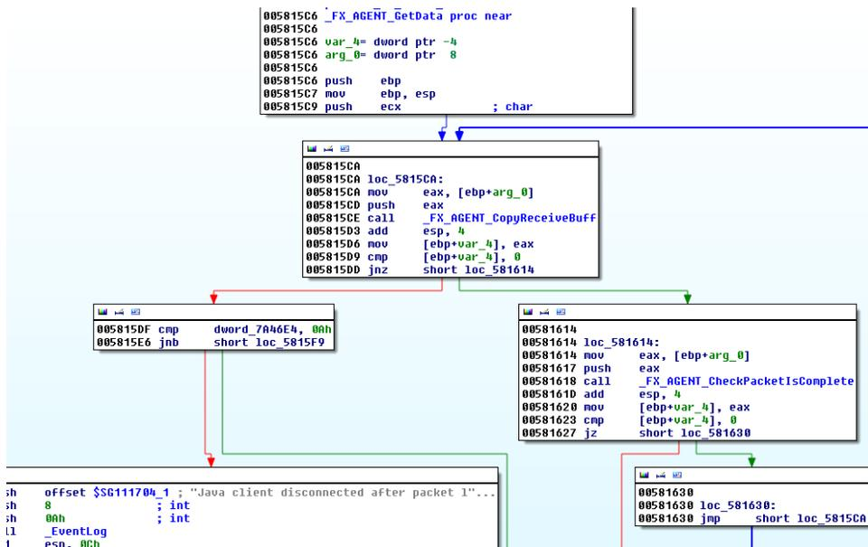
This time , our packet doesn't go to the function where Client Disconnected error logs located. We jump to loc\_581614 function. After we complete FX\_AGENT\_GetData function , we return to 0x00581320 address in FX\_Agent\_Cyclic function. After passing a few instructions in this function, we fall in a function which compares the first 4 bytes of our packet again;
